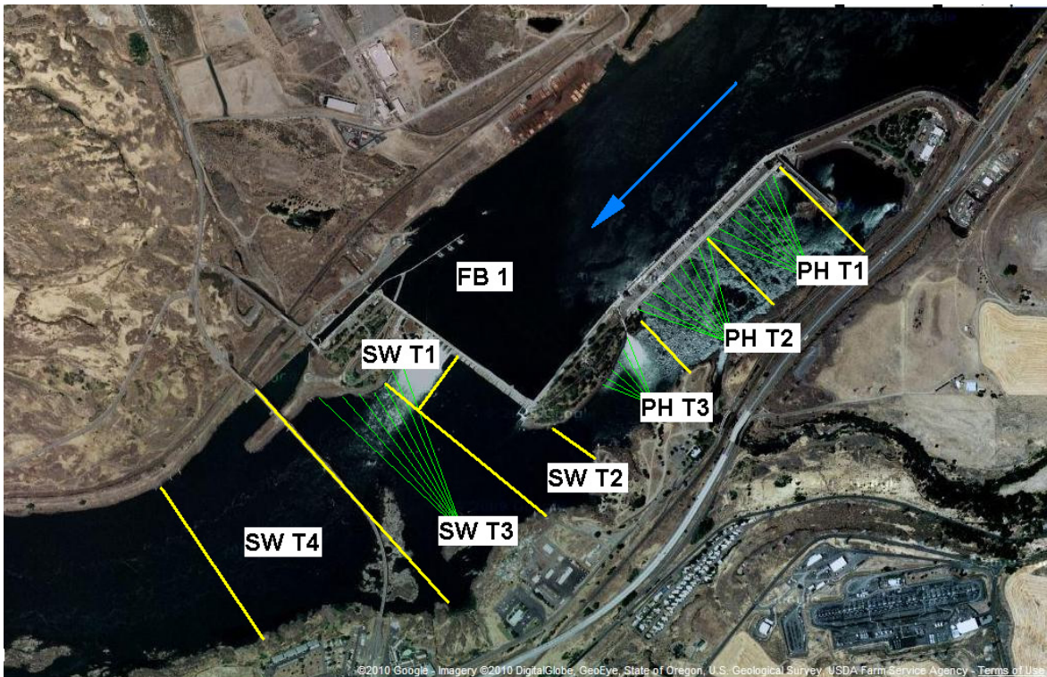
Figure 4. Image of The Dalles Dam at Columbia River mile 192 (©Google Images 2009). Flow is from right to left with the avian array represented by thin green diagonal lines and the observation zones demarked by yellow lines.
